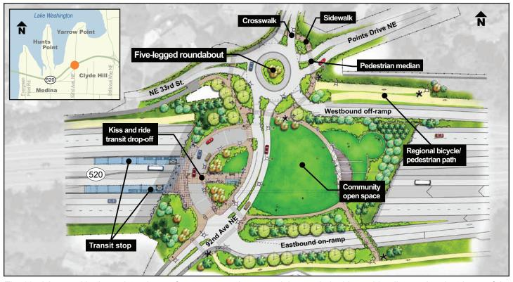
The 92nd Avenue Northeast interchange features a one-lane roundabout to help drivers, bicyclists and pedestrians safely and efficiently navigate local streets and the SR 520 highway off-ramp.
